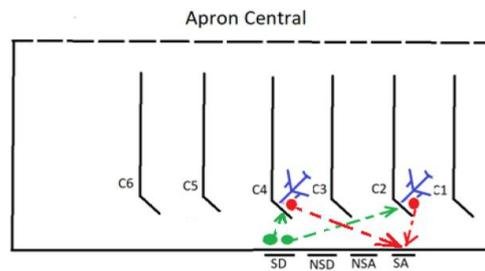
**Figure 1** Deployment scheme of aircraft operating the flights 2 and 3 on the apron
