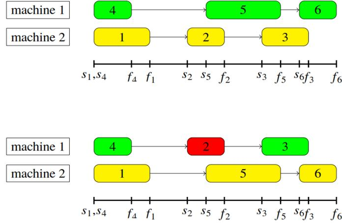
Figure 1 FIS schedules: two possible assignments of 6 jobs to 2 machines. If the machines are identical, both schedules are feasible. However, if job 2 cannot be processed by the first machine, then the second schedule is not feasible.
