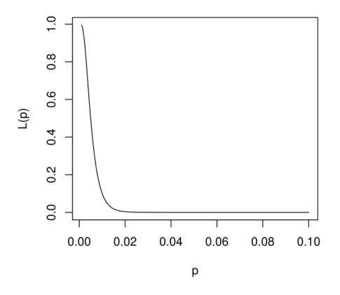
Figure 2 Operating characteristic curve of plan (26, 2.57768)
